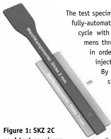
**Figure 1: SKZ 2C peel test specimen**
