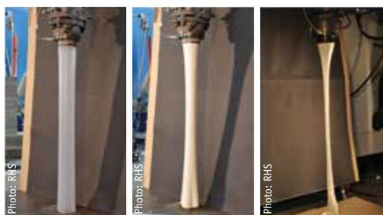
**Figure 1: Preform-formation in extrusion test**
