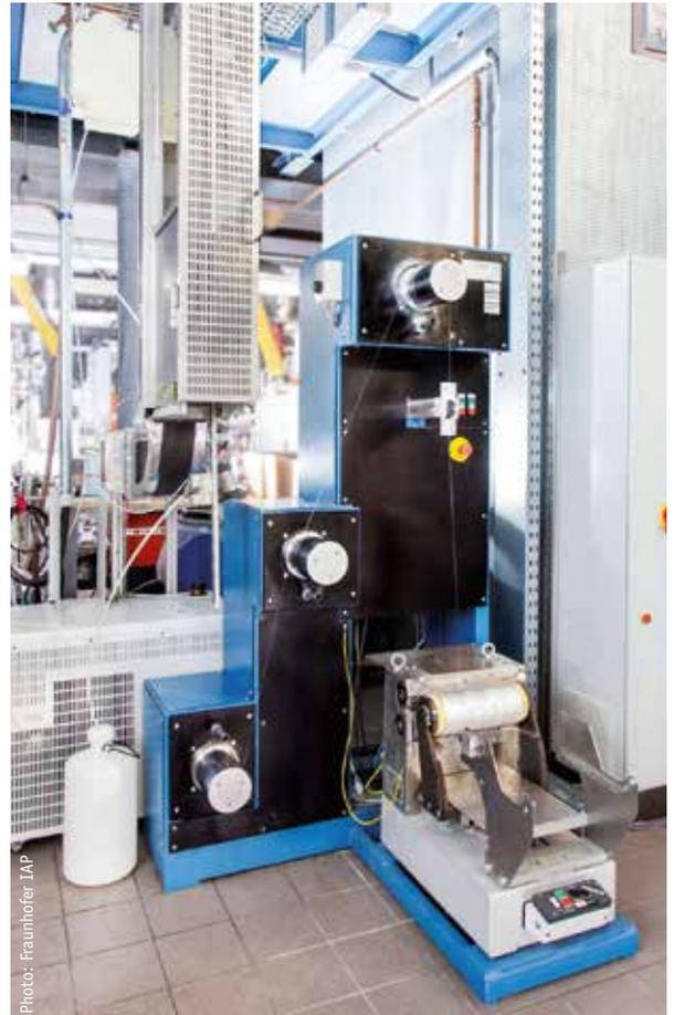
**Figure 2: Fourné melt spinning machine**
